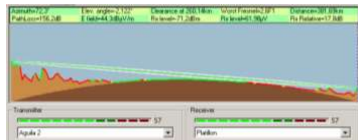
Fig. 2 Profile of the 382 km path between Pico del Aguila and Platillon in Venezuela
